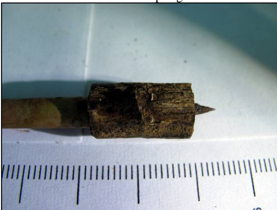
Striker 12 was badly corroded and seized; this would have prevented operation
