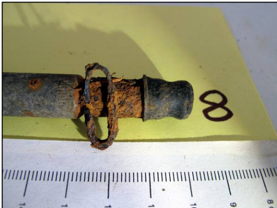
The retaining pin of fuze 8 was almost rusted through, but the striker was seized
