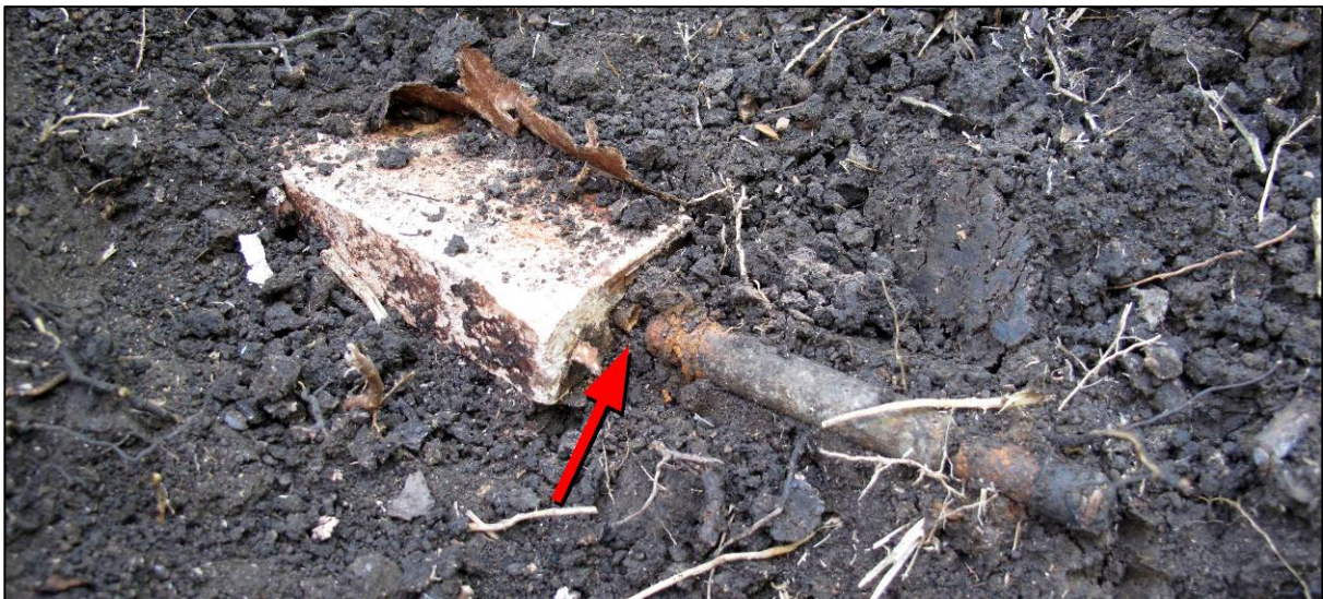
None of the wood casing remains from mine 6. There is a clear break between the fuze and the TNT block (indicated by the red arrow); this was filled with mud.
