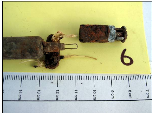
The retaining pin of fuze 6 was in relatively good condition
