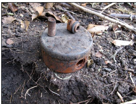
The PMN with detonator removed; in some mines the detonator could not be extracted
