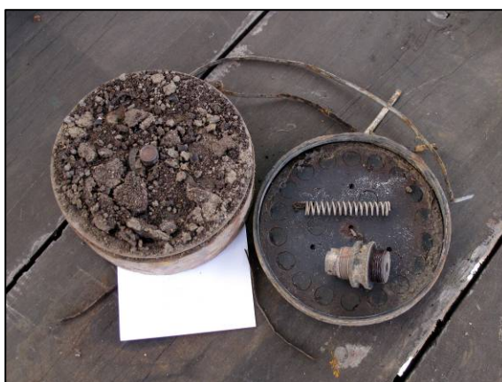
In some cases, soil had almost filled the void beneath the pressure plate
