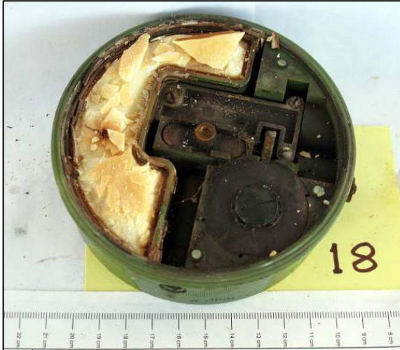
Top plate removed to show the main charge (to the left) which is in good condition. The fuze mechanism (to the right) has degraded
