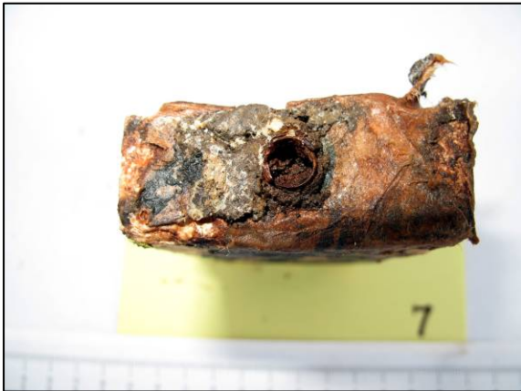
The end of the TNT block, looking into the mouth of the detonator tube
