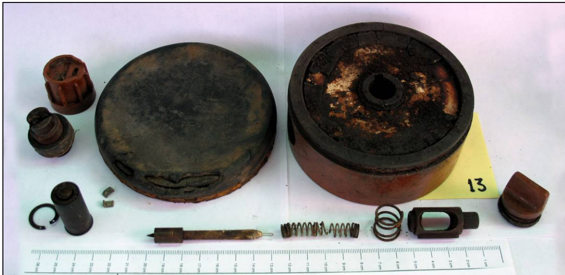
Components of mine 13 with TNT charge still in place within the body. The mine may have been functional despite the striker spring being badly deteriorated
