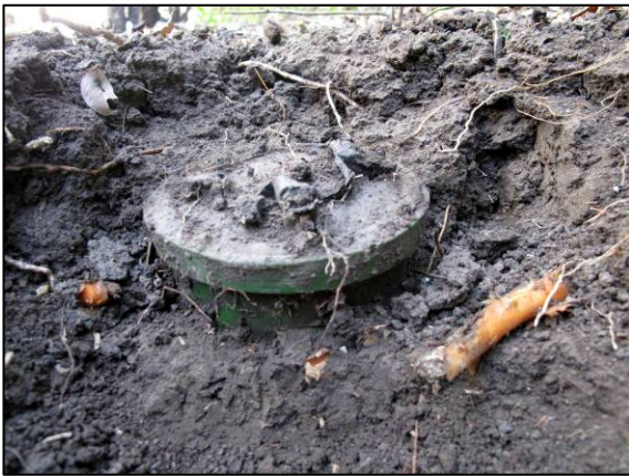
Deterioration of the rubber pressure plate cover
