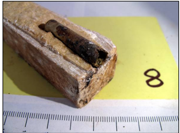
The TNT block broken open to show the corroded detonator tube
