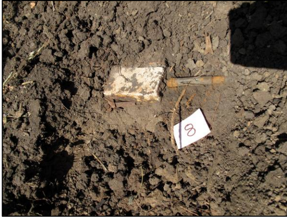
Every PMD-6 mine recovered had a break between the fuze and the charge
